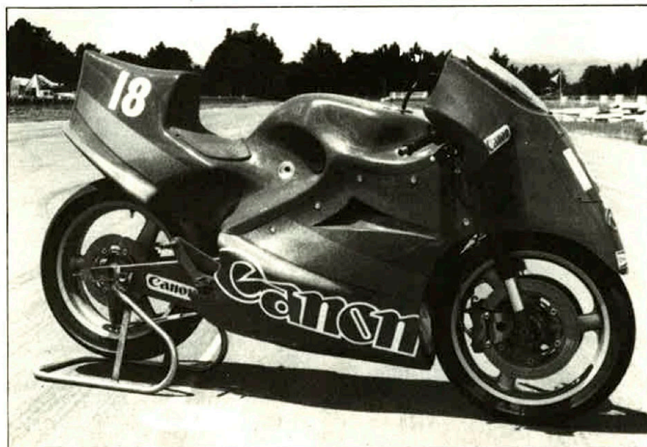
Bodywork and monocoque chassis are fashioned from kevlar and carbon fibre
