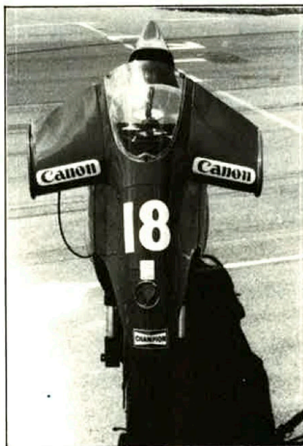
Twin aerofoils are one of the Denco designer's intuitive design ideas
