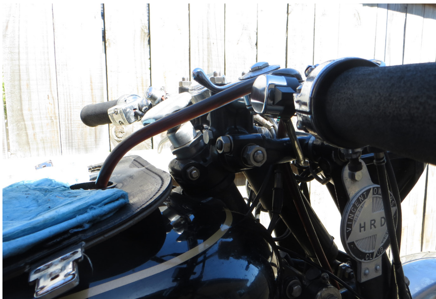
Plastic fantastic oil return bypass which worked - Phew!
