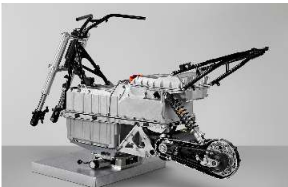
Innovative electric drive via drivetrain swing arm with liquid-cooled alternator, tooth belt and planetary gear
